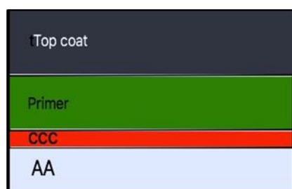
Figure 2: Schematic draw of a typical multi-coating system
