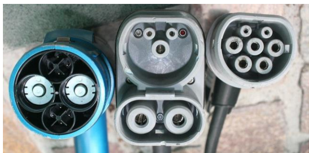
Picture 2: CHAdeMO, Combo2 and Type 2 chargers [8]
