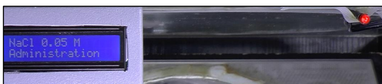
Figure 7: The LCD screen with the information of administration (left) and the LED light which shows the administration (right upper corner)
