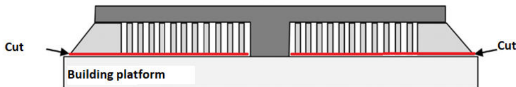
2. Figure, Position of the horisontal cut on the test specimen [10]
